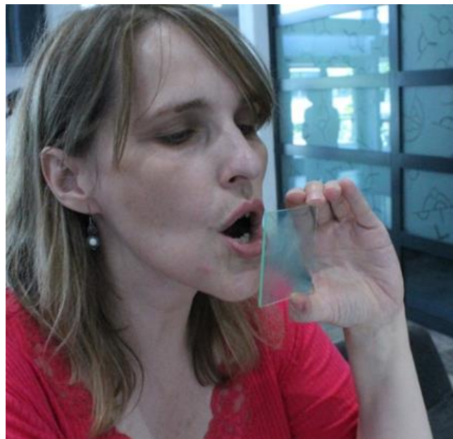
Figure 17. Finding the glass and emulsion side of a holographic plate – practice in the light!
