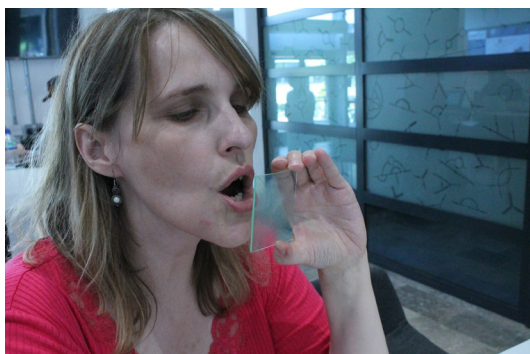
Breathe on the holographic plate to find the glass side that fogs up.
