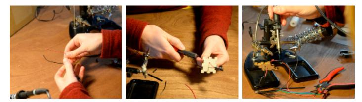
Insert the switches into the holes in the box. Secure the switches with nuts to the wooden box.
