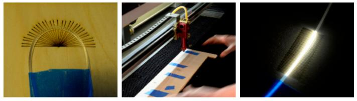
When removing the optical fibre from the shelve, make sure it stays curved, this to reduce the chance of breaking the fibre.
