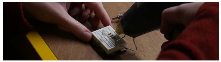
Connect the black wire of the battery conenctions to the GND (ground) leg of the white LED. Secure this connection on the electric board also with hot glue.
