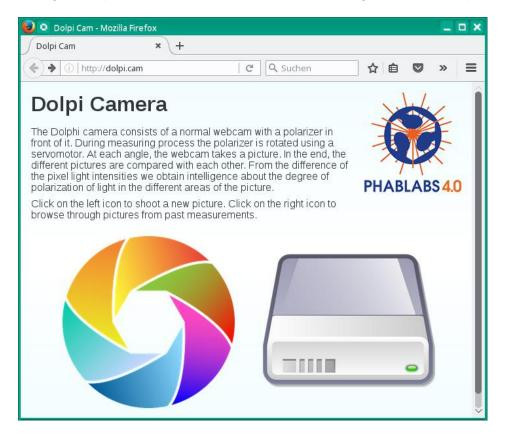
Click on the colourful shutter on the left-hand side of the browser window (only once). The servomotor should now begin to move and the webcam should take pictures. After the measuring process has finished, you should see the resulting photos in the browser.
