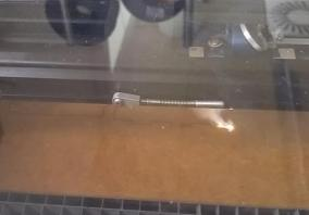
Now, the laser head will cut out the parts from the plywood sheet. Once finished, take the plywood out of the machine and try to assemble the different parts, at first without using glue. It should look like this:
