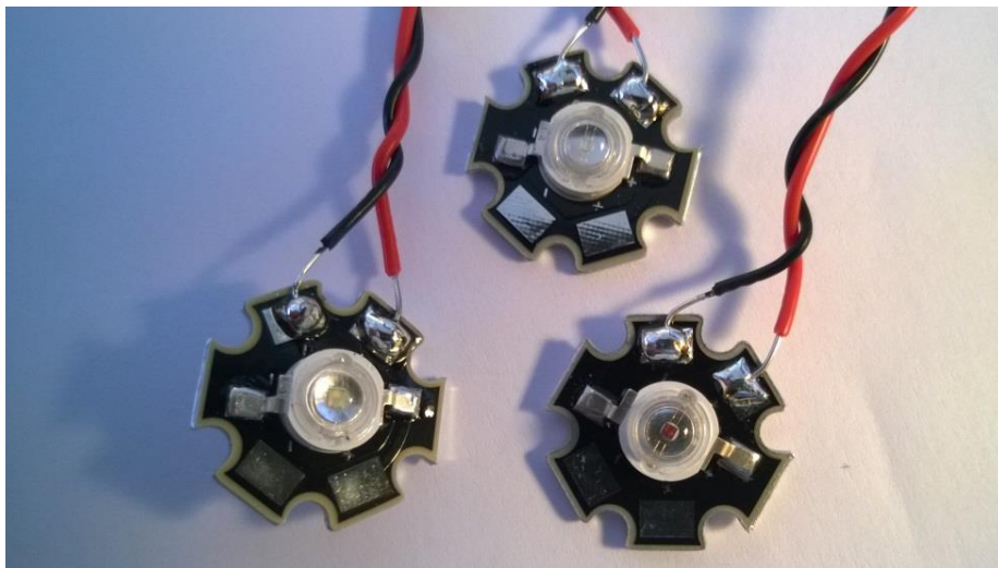
Figure 16: The three LEDs with their wires attached
